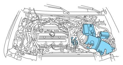
• Cover the highlighted areas to prevent water damage when cleaning the engine.
